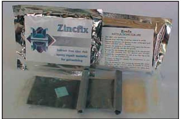
**Figure 8:** Zinc Fix consists of 100 grams of zinc rich epoxy. Once the activator is mixed the contents must be used within 30 minutes. Zinc fix was specifically developed as a site repair kit for galvanizing.
