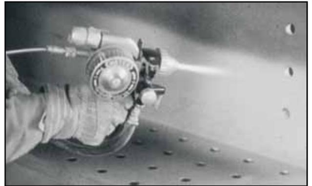
**Figure 7:** Zinc thermal spray is an ideal method of hot dip galvanising repair. Surfaces to be repaired must be cleaned and the zinc coating applied to  $30\mu\text{m}$  over and above that specified in terms of SANS 121 (ISO 1461: 1999).
