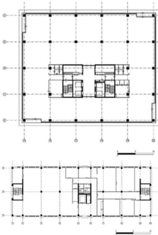
Figure 2 : Single corridor Slab and Central Core Plan <sup>15</sup>
